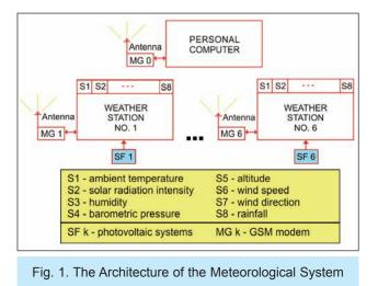
The data reading provided by the meteorological stations it is made in an order initially set via the acquisition program running on the personal computer (PC).
