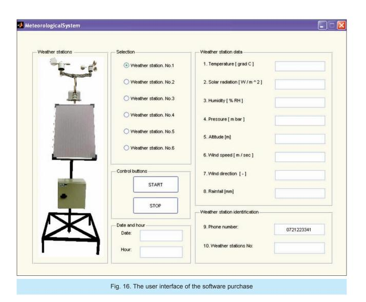
To view the latest values acquired, the interface has six radio buttons. Through these buttons, it can be selected at a time those six weather stations.
