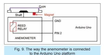
Pin 2 of the Arduino platform structure (see figure 9) is a digital input pin. Pin 2, in the application, is configured to trigger an external interrupt on a falling edge of the input pulse.
