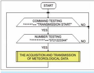
Fig. 14. The program flow diagram of the ATMega328P microcontroller constituent
