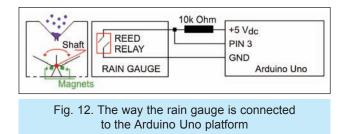
The pin 3 of the Arduino Uno platform structure (see figure 12) is a digital input pin and is configured as pin 2 in connection from the anenometer scheme (see figure 9).
