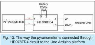
The A1 pin used for connecting the PYRA 04 pyranometer to the Arduino Uno platform is an analog pin. The Arduino Uno platform analogues pins are connected to an analog-digital converter that has a resolution of 10 bits.
