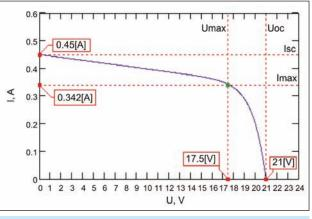
Fig. 3. Current-voltage of the photovoltaic panel TPS-103 characteristic
