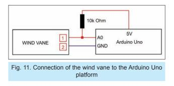
The A0 pin used for connecting the wind vane to the Arduino Uno platform, it is an analog one.
